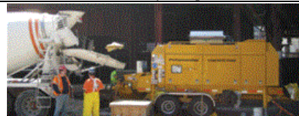
Capable of handling high psi and long distance pumping up to 1,000 feet vertically or 4,000 feet horizontally
