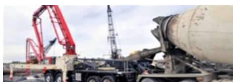
Mobile, truck-mounted boom pumps with vertical reach over 200 feet
