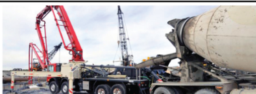
Mobile, truck-mounted boom pumps with vertical reach of over 200 feet Fleet Size: 617
